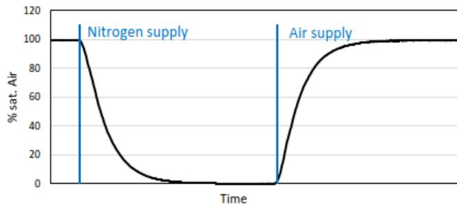
Fig.2. - Schematic illustration of the concentration change when using the DSM.
