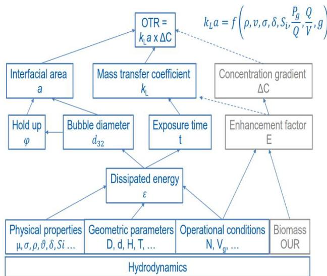
Fig. 1 – Correlation between OTR, the  $k_La$  coefficient and hydrodynamic parameters in a bioreactor. <sup>(8)</sup>
