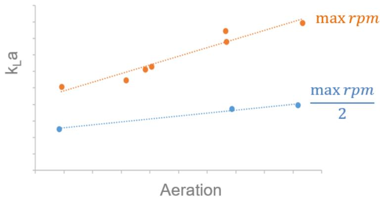
Fig.8. Influence of Power Input (agitator speed [rpm]) on the  $k_{La}$  value with increased aeration measured at the “sweet spot” of the fermenter
