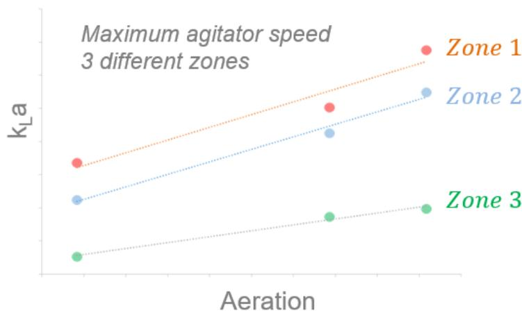
Fig.7. Spatial differences in the correlation of measured  $k_{L,a}$  with increased aeration and constant agitation speed.
