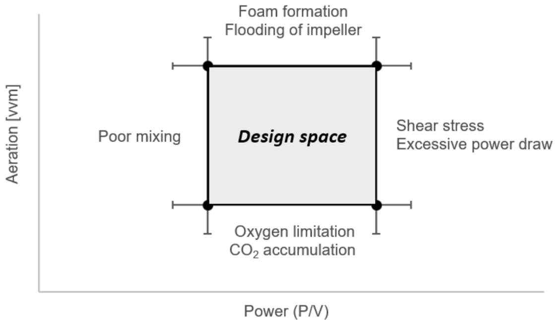
Fig.10. Defining the design space for the bioreactor characterisation
