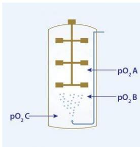
Fig.6.  $k_{L,a}$  measurement points within 12,000L bioreactor (type and position of sparger and impeller also shown).
