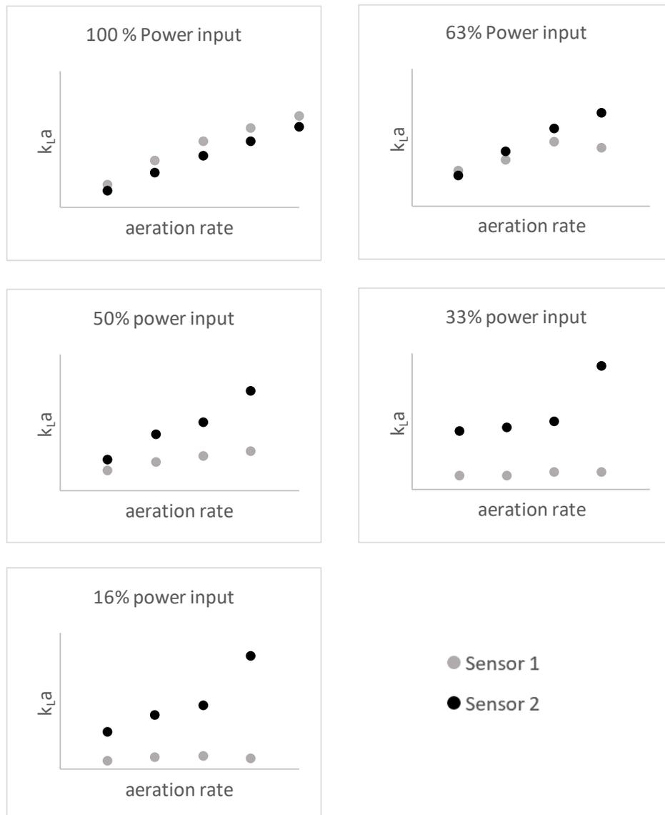
Fig.11. Experimental results showing different  $k_{L,a}$  values measured across a range of gassing rates and agitator speeds.
