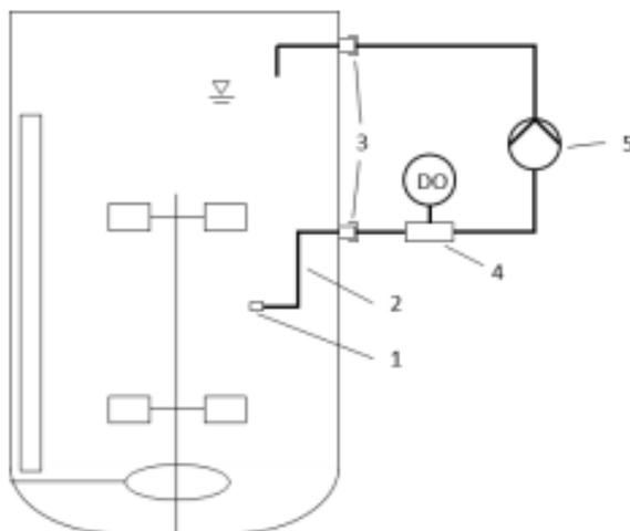
Fig.3. - Schematic illustration of the measuring method. (1) membrane and frit (2) sample inlet pipeline (3) Connector to the reactor (nozzle). (4) flow-through cell (5) peristaltic pump for sample return.
