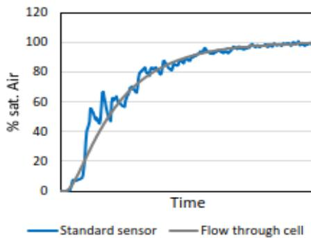
Fig.5. Comparison of sensor readings when comparing the standard and flow-through cell methods.
