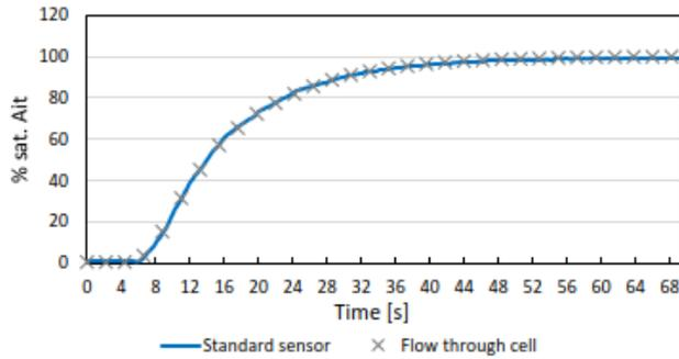
Fig.4. – Oxygen concentration curves comparing the standard method with that of the flow-through cell.
