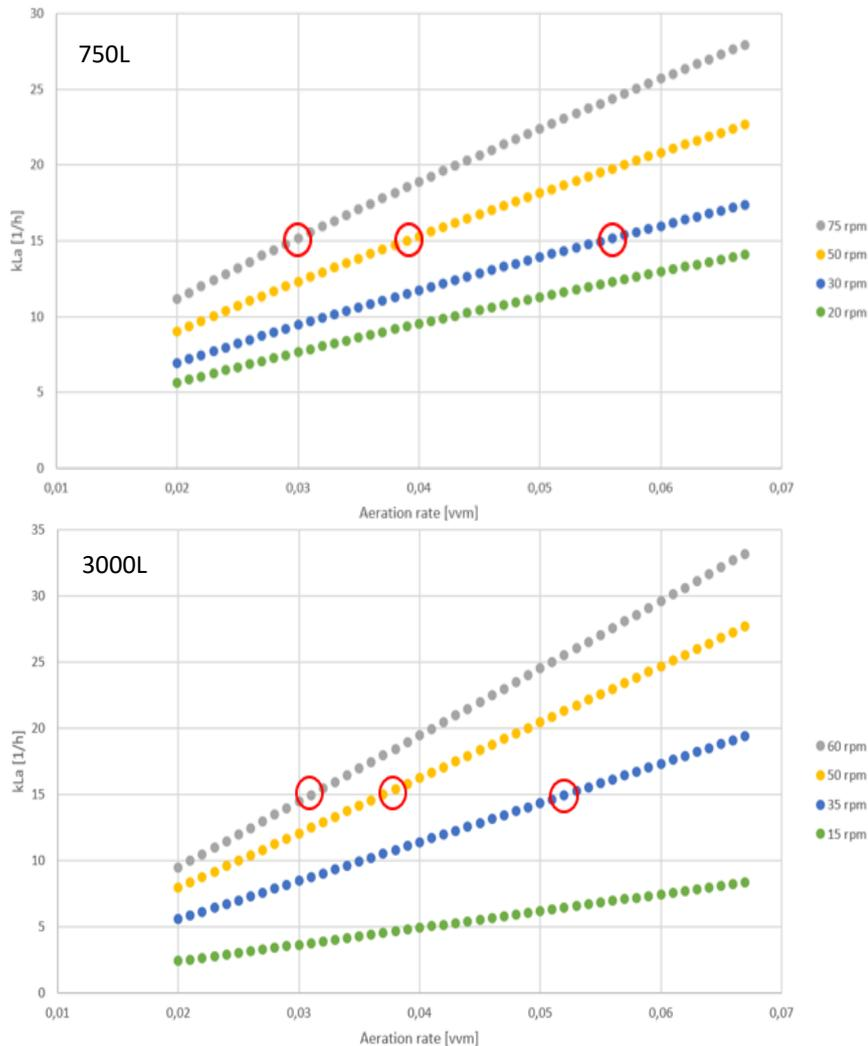
Fig.13.  $k_{La}$  values predicted against increasing aeration rates for varying agitator speeds in 150, 750 and 3000L bioreactors.
